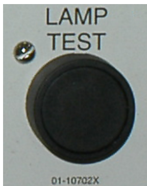
Figure 8. Lamp Test Switch
