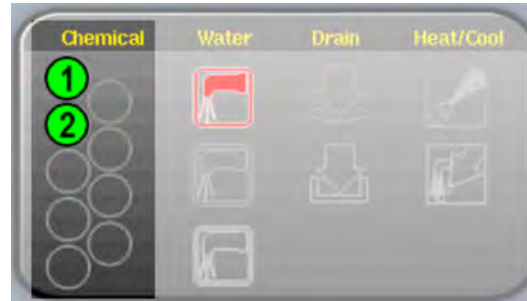
Figure 12. Chemicals from Valves 1 and 2 Injecting
