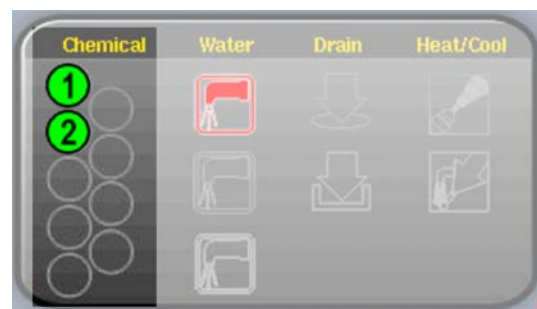
Figure 12. Chemicals from Valves 1 and 2 Injecting
