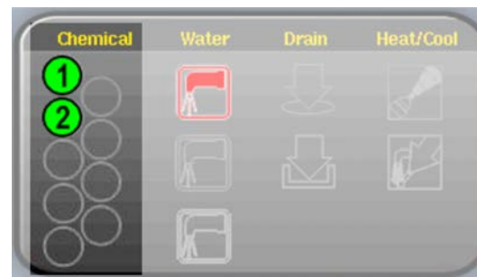
Figure 10. Chemicals from Valves 1 and 2 Injecting
