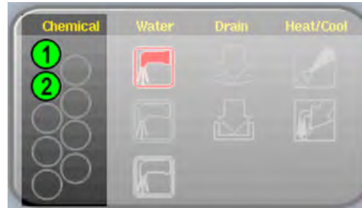
Figure 11. Chemicals from Valves 1 and 2 Injecting
