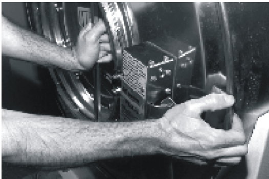
Figure 4: Hold Door Shut when Testing the Door Latch Interlock
