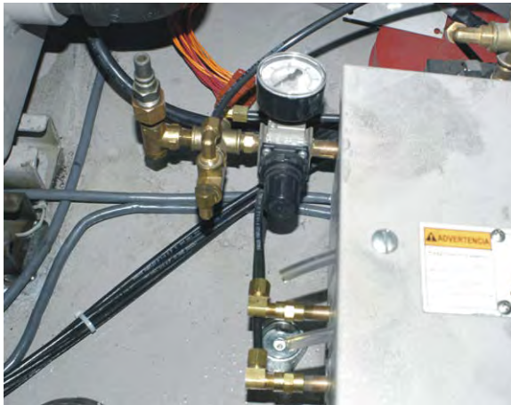
Figure 14: Air Pressure Gauge and Regulator on Top of Top Plate for Discharge Door
