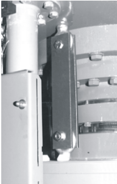
Figure 4: Safety Stands for 1-station Press Models (deployed shown at left, stowed shown at right)
