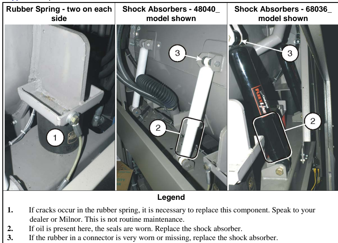
Figure 15: Suspension Components on Each Side of Rubber Spring-resting Washer-extractor (see Supplement 3)
