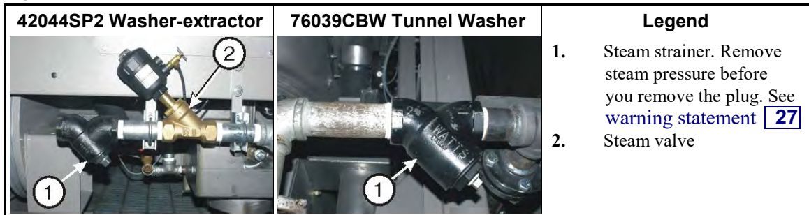
Figure 14: Steam Inlet Strainer. These are examples. Your machine can look different.
