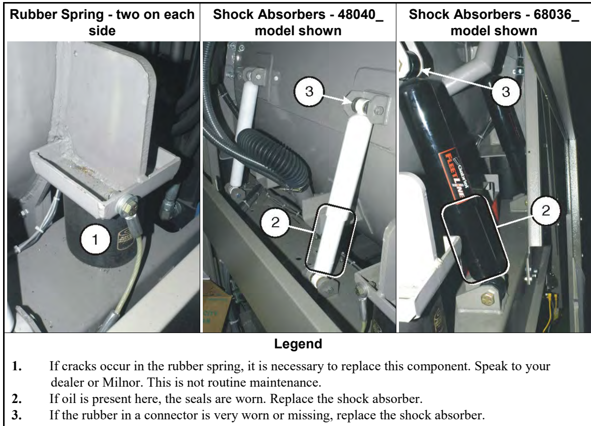
Figure 22: Suspension Components on Each Side of Rubber Spring-resting Washer-extractor (see Supplement 4)
