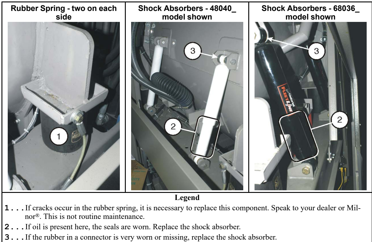
Figure 20. Suspension Components on Each Side of Rubber Spring-resting Washer-extractor (see Section 3.3.2 : About the Shock Absorbers, page 33)
