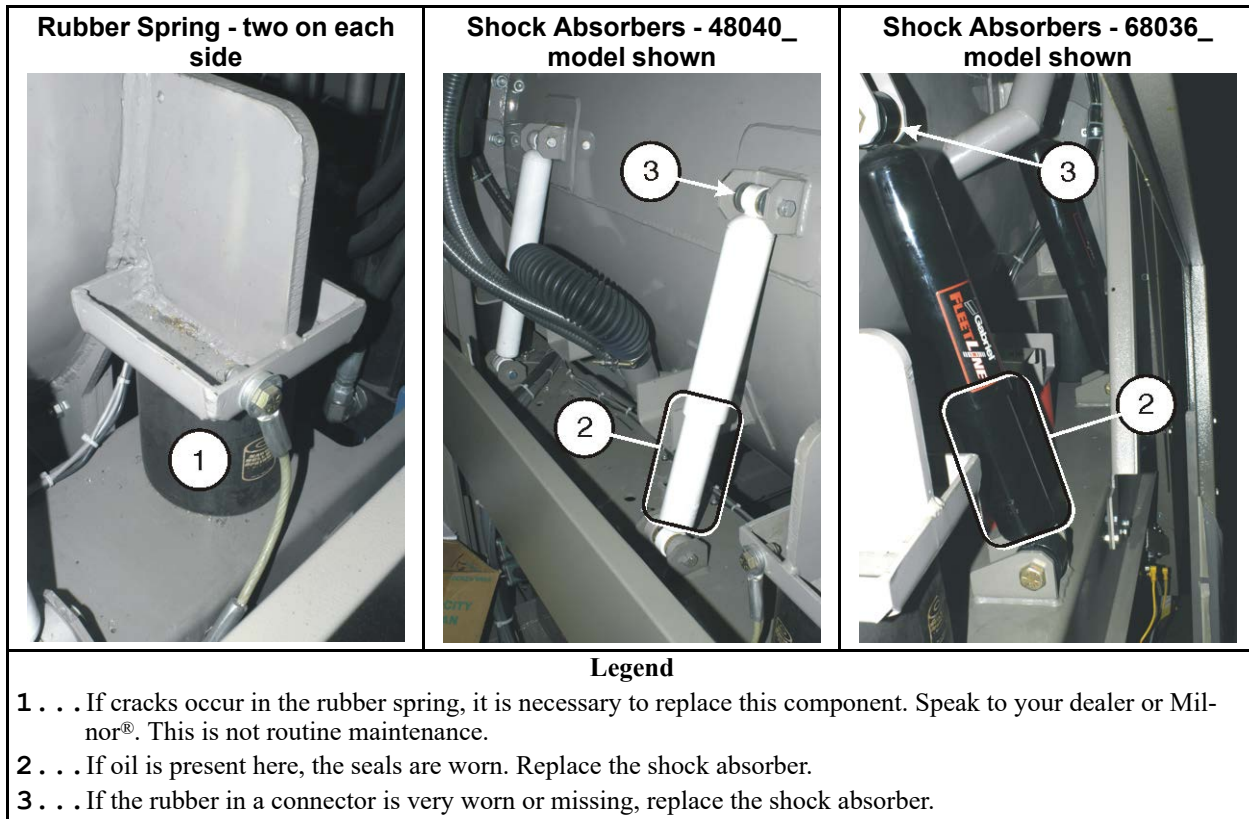
Figure 23. Suspension Components on Each Side of Rubber Spring-resting Washer-extractor (see Section 3.3.3 : About the Shock Absorbers, page 35)
