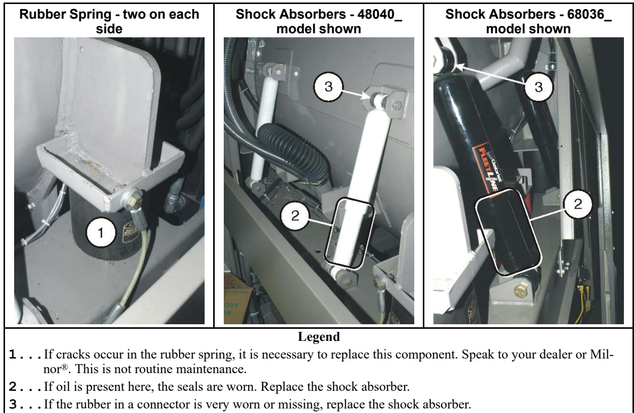
Figure 23. Suspension Components on Each Side of Rubber Spring-resting Washer-extractor (see Section 3.3.4 : About the Shock Absorbers, page 36)
