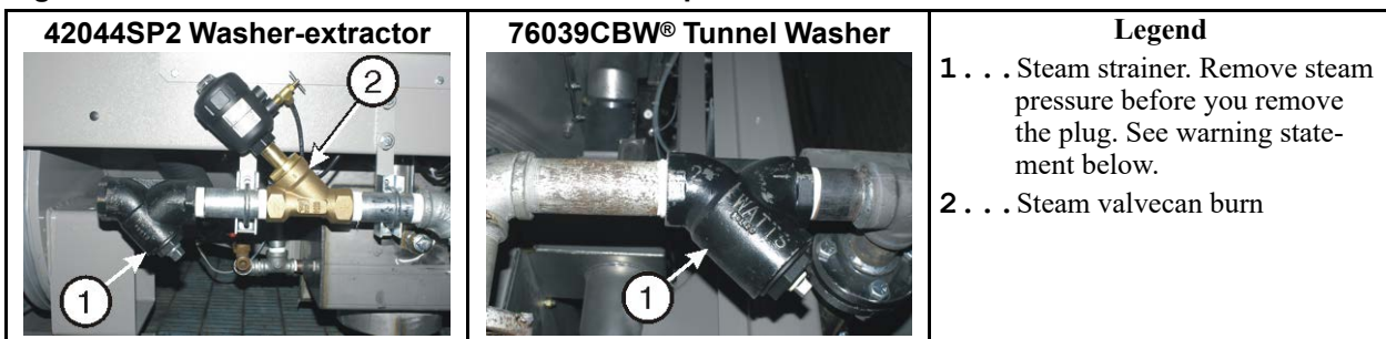
Figure 13. Steam Inlet Strainer. These are examples. Your machine can look different.
