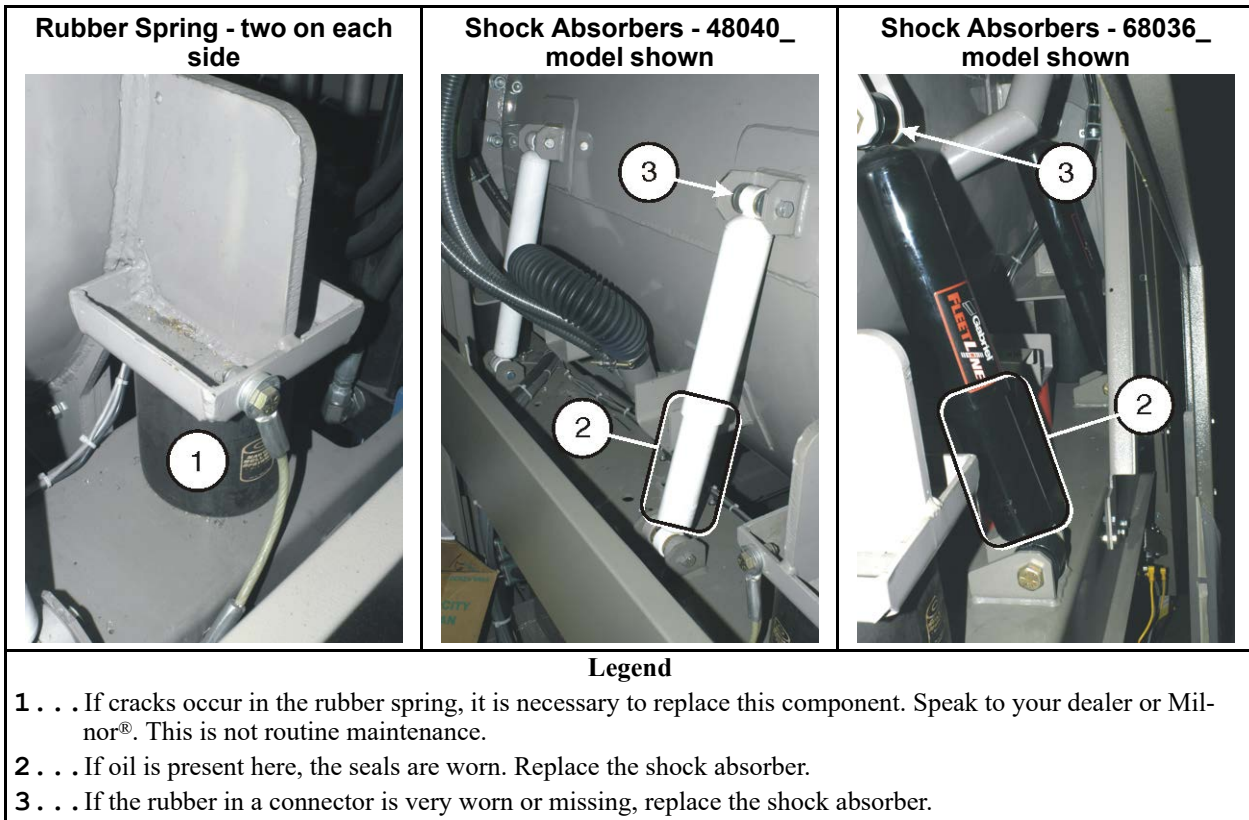
Figure 24. Suspension Components on Each Side of Rubber Spring-resting Washer-extractor (see Section 3.3.4 : About the Shock Absorbers, page 40)
