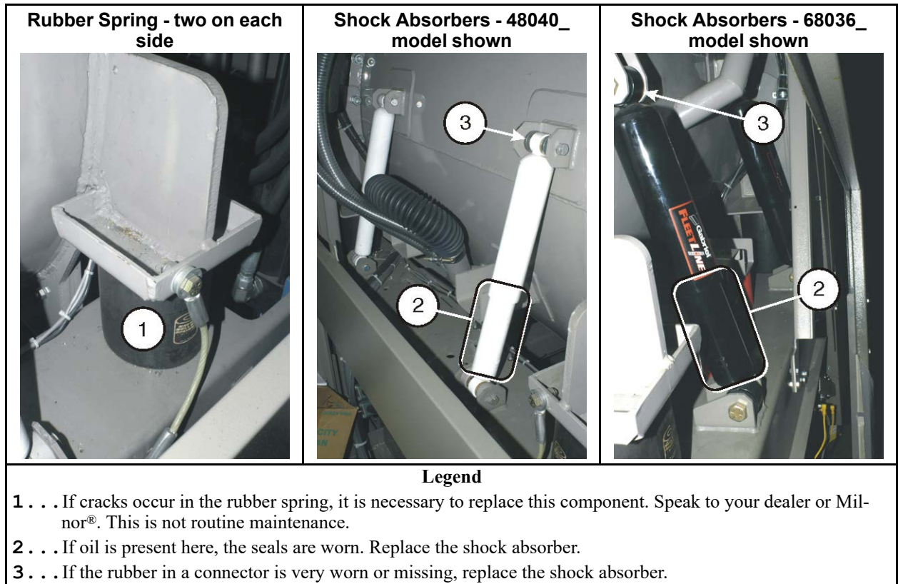
Figure 24. Suspension Components on Each Side of Rubber Spring-resting Washer-extractor (see Section 3.3.4 : About the Shock Absorbers, page 40)
