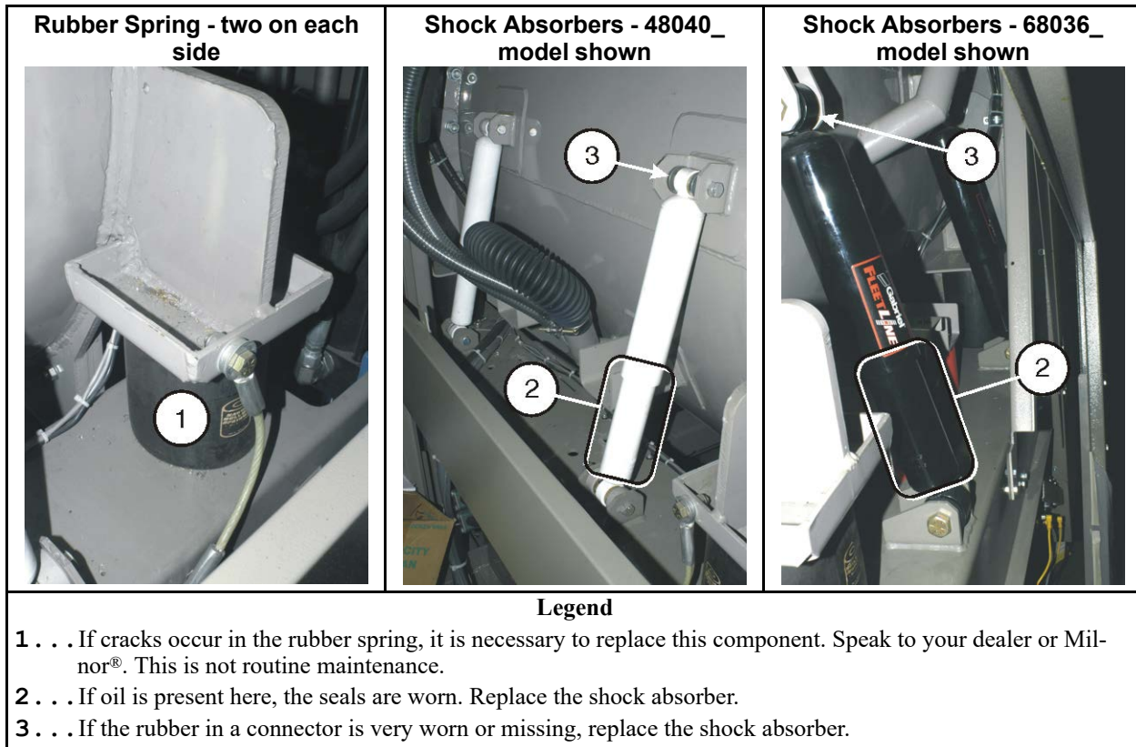
Figure 24. Suspension Components on Each Side of Rubber Spring-resting Washer-extractor (see Section 3.3.4 : About the Shock Absorbers, page 37)
