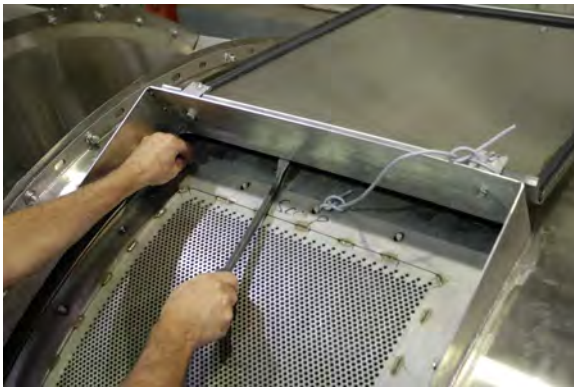
Figure 1: Removing Inner Hatch Nuts (G3 CBW shown. G4 similar.)
