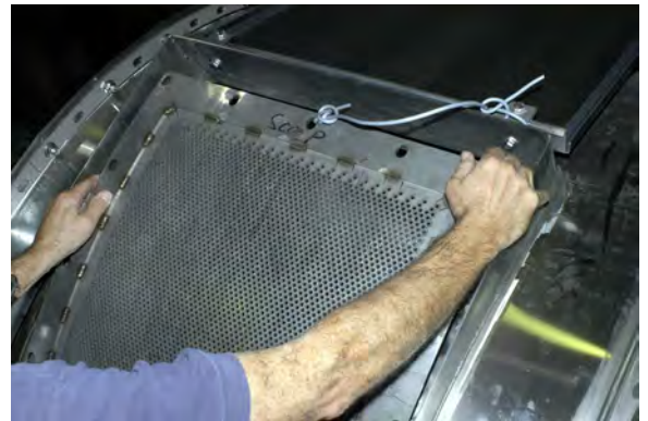
Figure 2: Lifting Off Inner Hatch (G3 CBW shown. G4 similar.)
