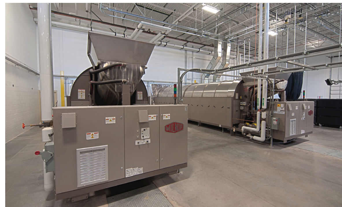
BELOW: Texas Healthcare Linen General Manager JoeMax Tomlin described the two Pellerin Milnor tunnels shown below as the “heartbeat of our operation.” These 8-module, 150 lb. capacity tunnels process hygienically clean textiles at a highly efficient rate of 0.4–0.5 gallons per pound.
