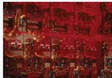
Testing electronics (up to 200 hours burn-in).
