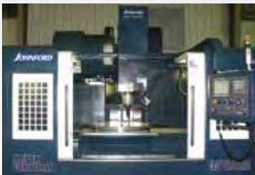
Vertical machining center creates larger parts in one clamping.
