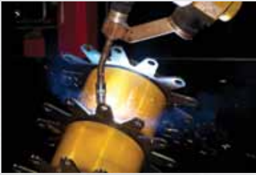
Robotic welder maximizes efficiency.
