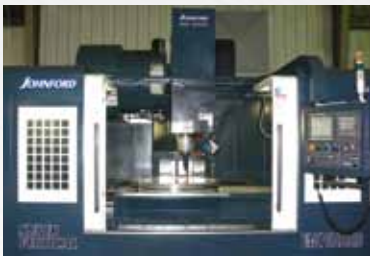
Vertical machining center creates larger parts in one clamping.
