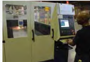
Laser Cutting yields greater use of raw material.
