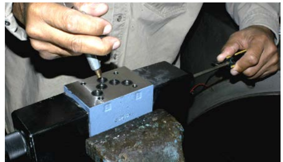
Figure 44: Bench-testing a Directional Valve
