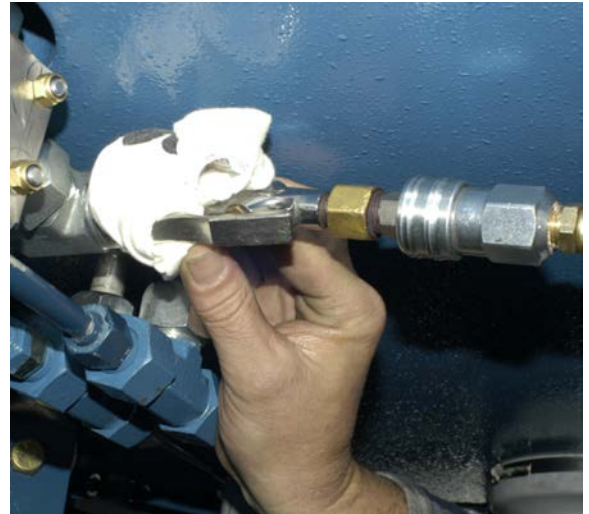
Figure 13: How To Apply Air Pressure to Seals
