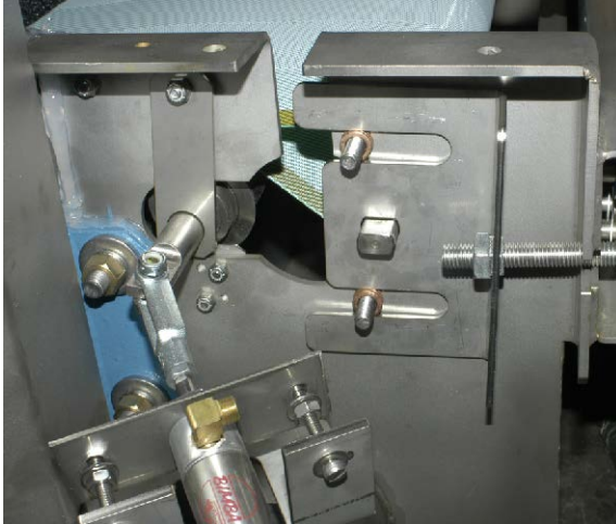
Figure 23: Tracking Bracket and Related Components Hanging from Tracking Roller
