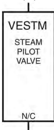
Figure 19: Electrically Operated Valve (VE)
