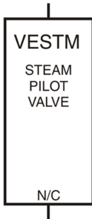
Figure 19: Electrically Operated Valve (VE)
