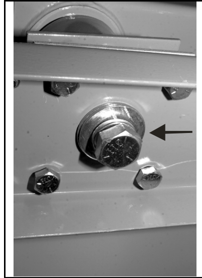
Figure 7: Shims stored under the mid frame
