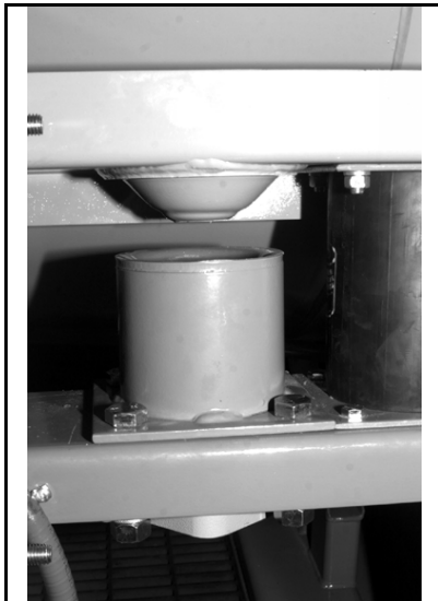
Figure 6: Cup weldment when setup for operation
